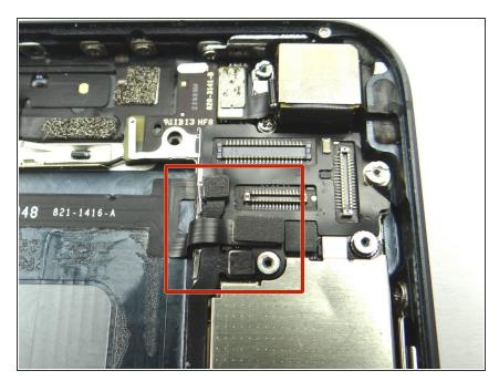
Reseat the bottom cable first, middle cable second and top cable third.
