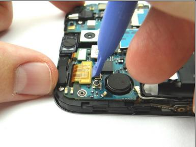
Use the Blue Pry Tool to disconnect the seven ribbon cable connectors on the logic board.
