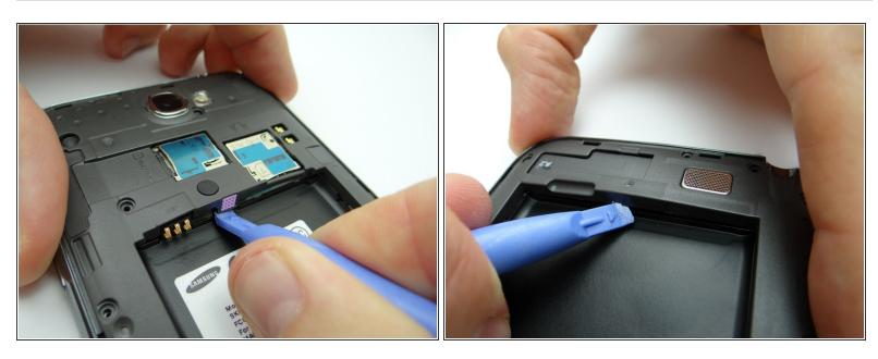
Pictures 1 & 2: Use the Blue Pry Tool to free the clips on the bottom and top of the battery holding area.
