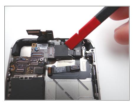
Wedge the flat end of the black spudger under the wi-fi antenna connecter and gently lift to release from logic board.
