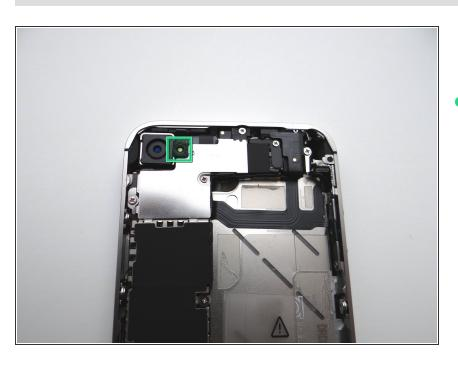
Use a pair of tweezers to remove the outer plastic ring (if present) located on top of the rear camera's flash. Place in COMPARTMENT B.
