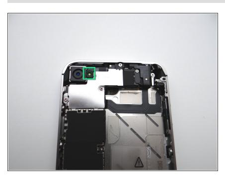
From COMPARTMENT B, if present, replace the outer plastic ring located on top of the rear camera's flash.
