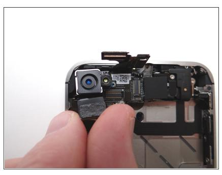
Remove the Rear Camera with your fingers. Place in COMPARTMENT C.
