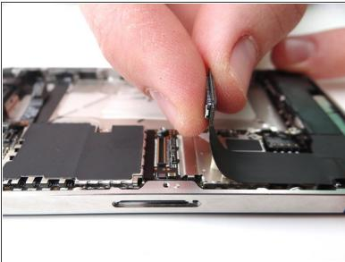
Fold the charging port assembly cable back into position and reconnect it to its socket on the logic board.
