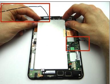
Replace battery from ZONE V. Make sure the antenna cable & lower speaker cable don't get trapped underneath.
