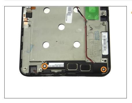
Replace two 3.1 mm #00 Phillips screws from SLOT 7.
